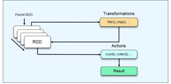
Transformations perform various operations and create new RDDs as a result. Actions come as a final step after completed modifications and return a non– RDD result (such as the total count) from the data stored in the R2 Driver.
